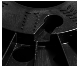
12. If you use manual winders, you can have holes to lock the cable end quickly and efficiently.
