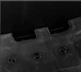
5. Two-way starting hole. The operator does not need to turn the drum in the machine. The operator can start from both sides.
