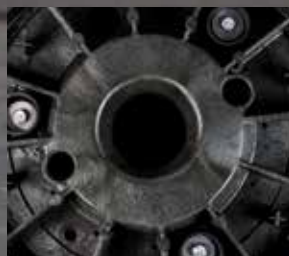
10. To reduce the risk of a stoppage in the winding equipment, our HD drums are made with a draft in the centre hole. This draft also increases the life span of the drum.
